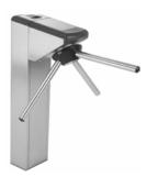
The column is available in two finishes: brushed stainless steel (AISI 304) or 1020 carbon steel with black or beige epoxy powder coating. It features fully rounded corners and a smooth surface with no exposed screws, in addition to a reinforced internal structure and plenty of space for practically any access control solution. It also has room for a no-break power supply unit and a card collection box (not included).
