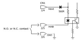
Turn-enabling through tension pulse is shown in the following figure. DC polarity must be observed. For high voltages, use an external resistor (110 to 220 V).
